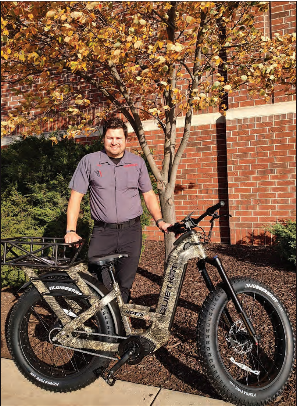
The electric bike is quieter and easier to transport than an ATV but more fun and less effort than a plastic sled when moving deer. This $4,000 QuietKat HD e-bike features a 1000-watt motor with two-speed internal gearing and a 15 amp hours battery that can move up to 28 mph and go about 25 miles of riding on a charge, according to Taylor Bentz, bike and service shop leader at Scheels in Appleton. These beefy bikes also can be used with special wheeled trailers to move deer, tree stands and other hunting gear.
