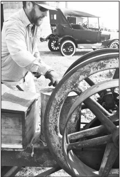
Greg Senn fuels up his 1911 Galloway fly-wheel engine, a five-horsepower, horse-drawn implement that powered a variety of devices a century ago. The engine retailed for $130, the equivalent of about $3,500 today.
