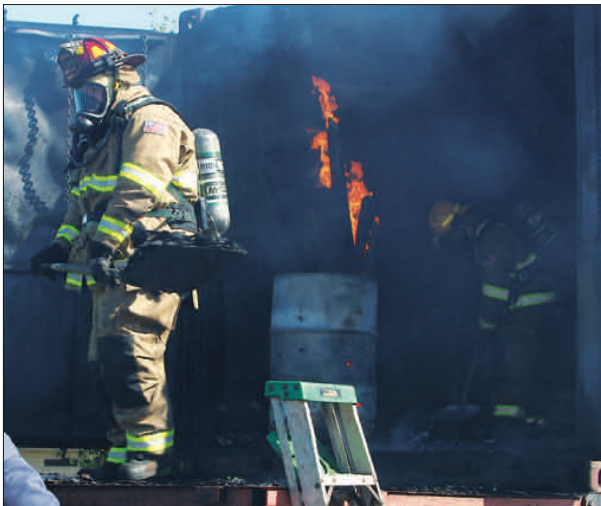
Lt. Robbie Woldt Jr., Bonduel Fire Department, is framed in the upper tier of a two-tier trailer designed to help firefighters recognize and survive flashover, a potentially deadly situation. He was among members of the Bonduel, Keshena and Shawano departments taking the training from Northeast Wisconsin Technical College in Shawano on Sept. 28.
