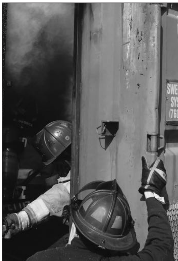
Controlling airflow is critical to efficiently putting out a fire. Del Zuleger, a Northeast Wisconsin Technical College instructor, consults with another faculty member at the door of the flashover simulator on how far to keep the door open and promote one of the four stages of a fire leading to flashover. DAVID WILHELMS
