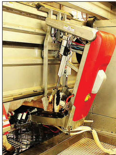
Twelve robotic milkers run around the clock to milk more than 1,500 cows at Strassburg Creek Dairy. The automated milking machines are one of the recent improvements on the Shawano County farm.
