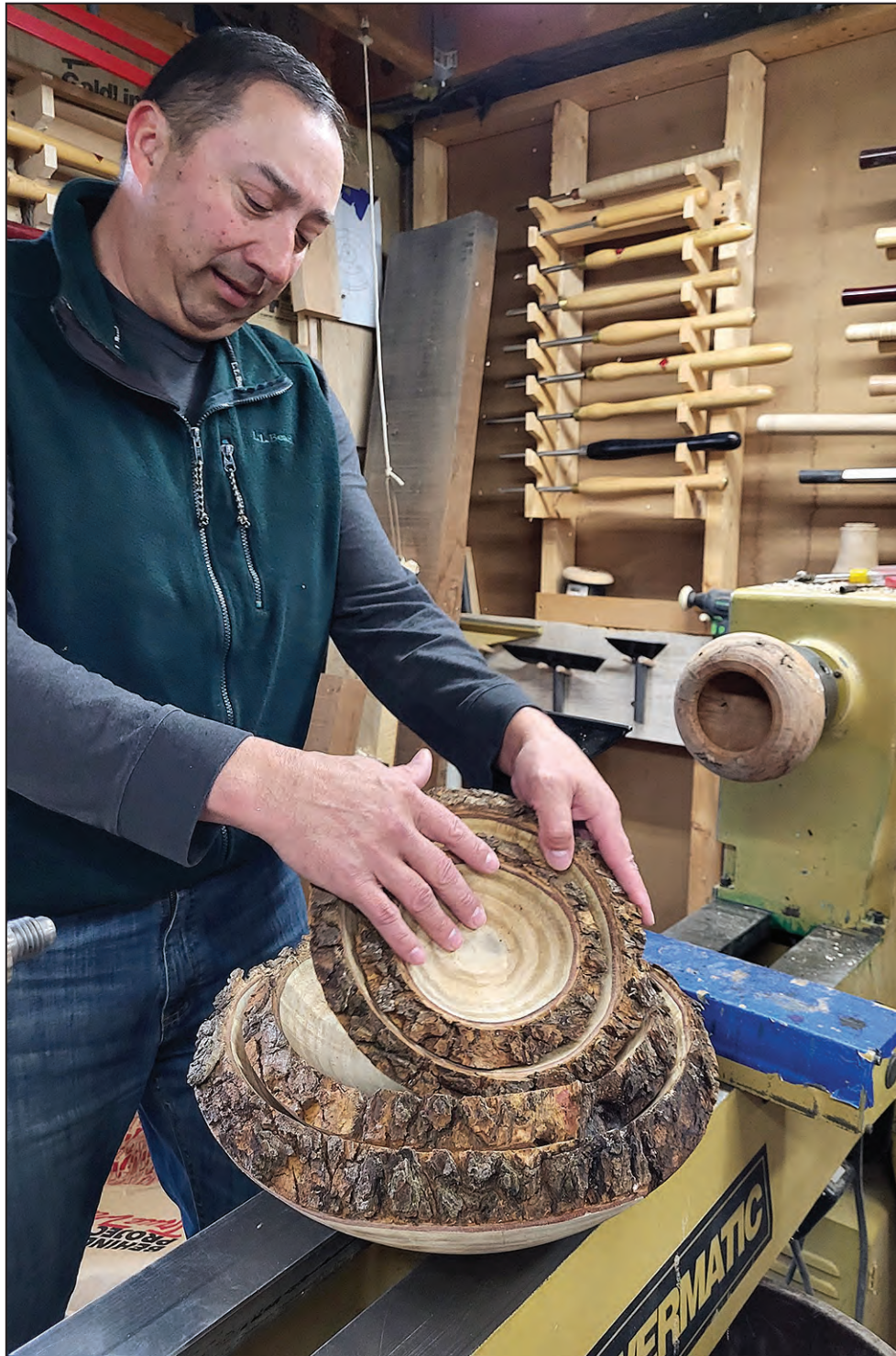
Local wood-turning artisan Jeremy Pyatskowit shows how a coring technique can turn a cherry burl into four nesting bowls. He will complete these bowls with a live edge on the large lathe displayed here. LYNN ZAFFRANN
