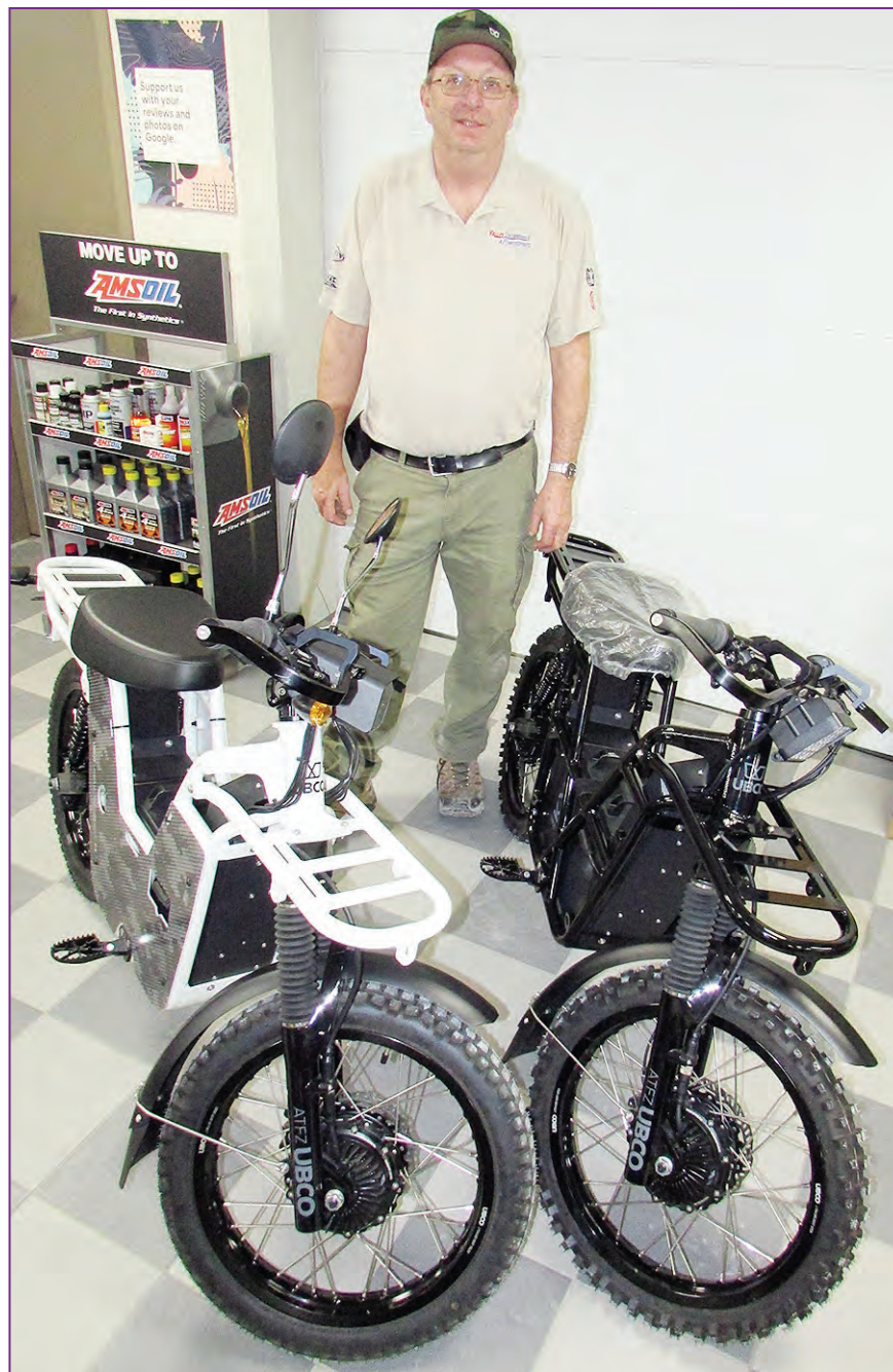
Lon Tesch, owner of Valley Snowmobile and Powersports in rural Hortonville, shows off the Adventure, left, and Work versions of the UBCO electric motorcycle. These 150-pound electric two-wheelers feature direct drive in both wheels, a 30 mph maximum speed and 30-pound batteries for up to 75 miles of range on a charge. They are classed as mopeds in Wisconsin and require only a driver's license to ride with no noise or fumes.
