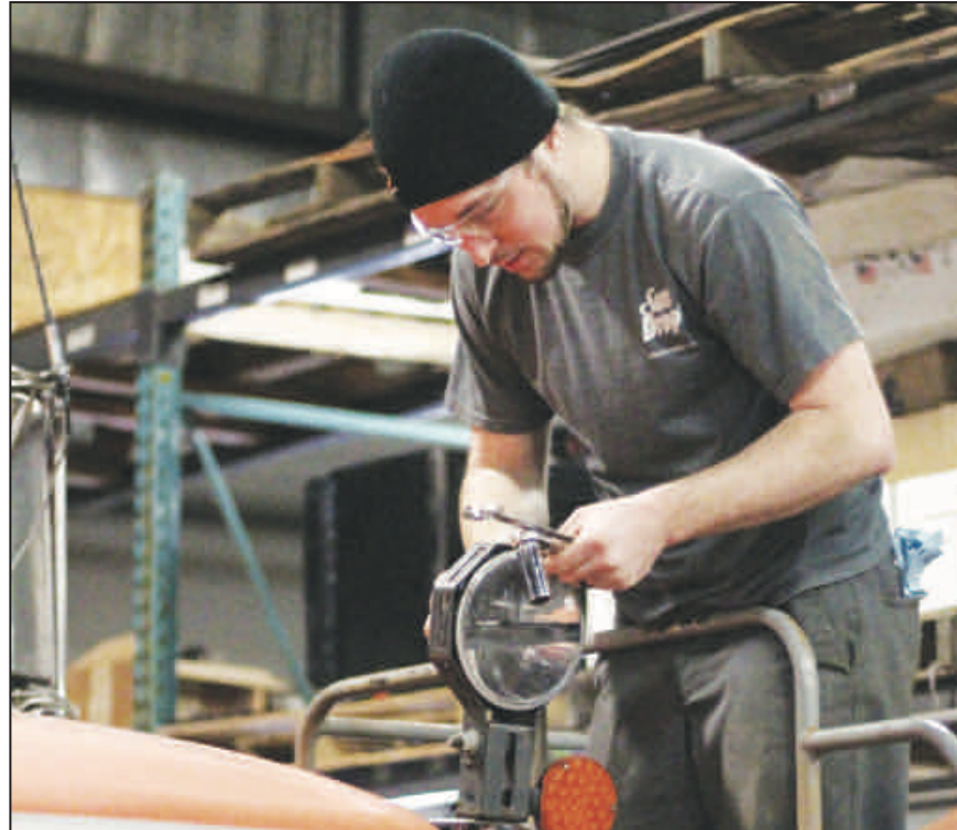
Garrett Smith, Shawano County Highway Department mechanic, replaces a light on one of the county's snowplows. Lights are one of ongoing maintenance in the winter, along with snowplow blade edges and “shoes,” said Grant Bystol, county highway commissioner.
