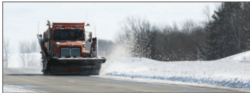
A Shawano County Highway Department snowplow cleans up a shoulder after the snowfall of Feb. 17 on state Highway 29. Trucks assigned to the four-lane highway are transformed each fall from their summer construction configuration to a snowplow with an “underbody” plow, a left wing plow, a right wing and the conventional front plow.
